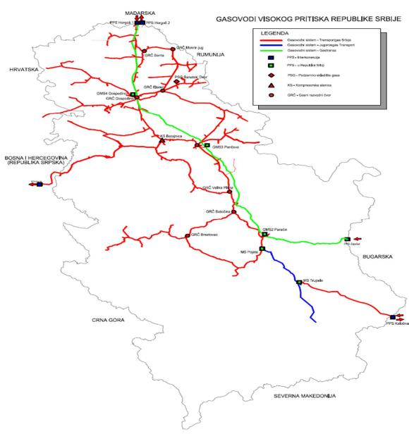
The length of the transmission system which is operated by the *Transportgas Srbija d.o.o. Novi Sad* amounted to 2,604.0 km on January 1, 2024. Out of the number, main gas pipelines account for 600.9 km, supply pipelines from local gas fields account for 176.8 km and distribution gas pipelines account for 1,826.3 km.
